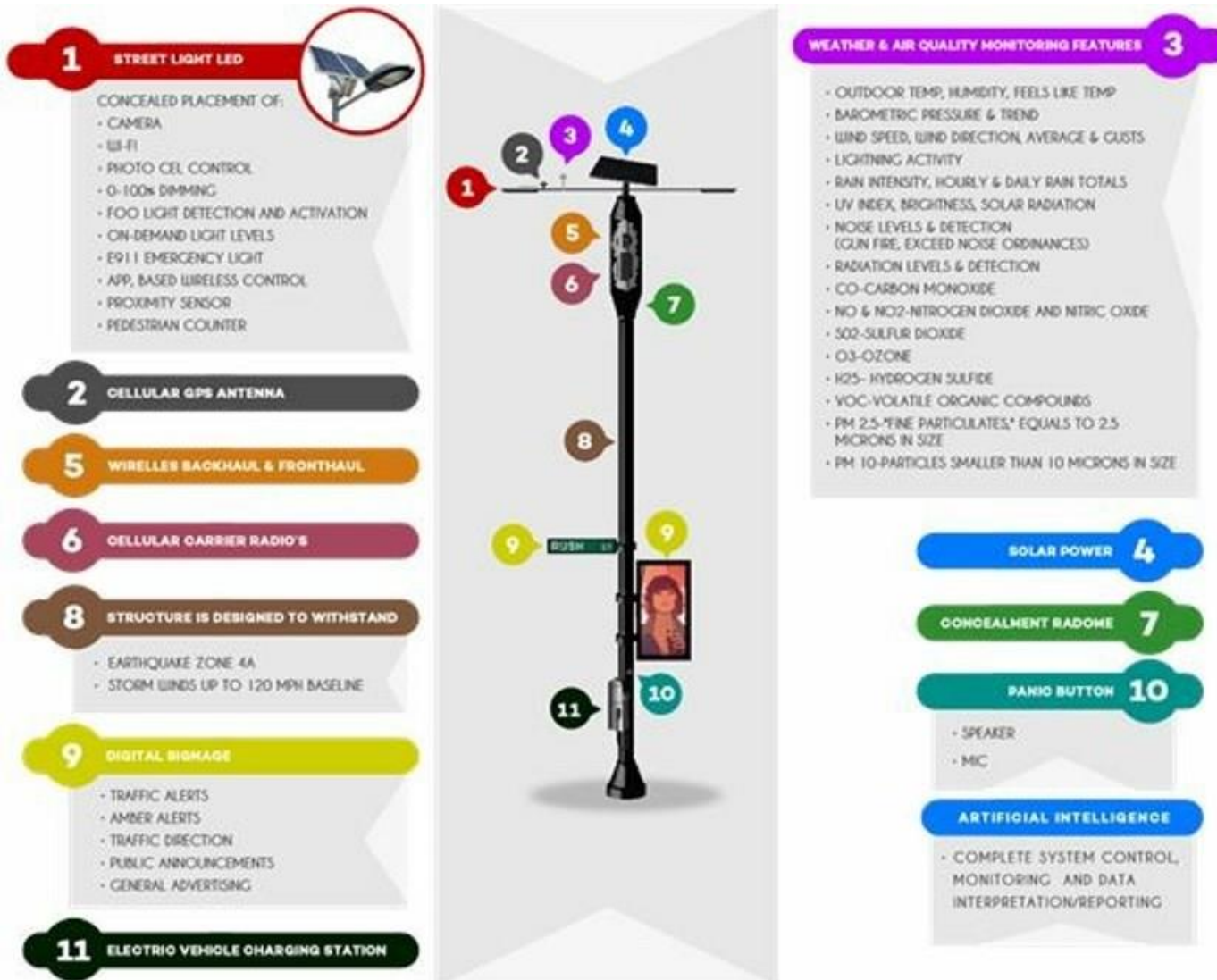
5G Street Light, Electronic Communications Package, and Weather Station – mummyanglais.wordpress.com
