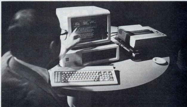
The IBM personal computer (Box 1328, Boca Raton, Fla. 33432), and printer as shown here. Other options, such as memory and graphics, are added with internal circuit boards.
